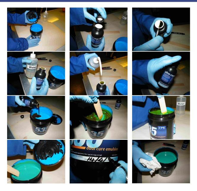
**#ScreenprintingTopTip:** Sensitise the emulsion at least 24 hours before it is needed in production to allow the Diazo to dissolve completely and for the emulsion to de-aerate.
