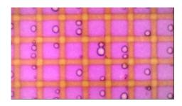
**#ScreenprintingTopTip:** Quite small variations in the depth of the emulsion in the coating trough can have a significant impact on the coating thickness. Where coating thickness is critical, i.e. four-colour halftone printing, ensure that the troughs are always filled to the same depth for each screen in the set.
